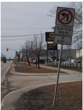
The intersection of Ellice WB at Berry uses a near side no left turn sign and has an advance warning sign.
