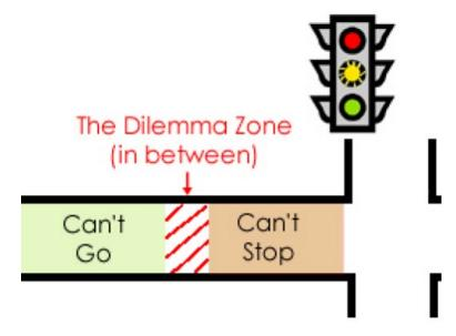
A yellow signal must allow a motorist to either come to a stop or proceed into an intersection before the red. Improper timing creates the dilemma zone. This is the zone where drivers are unable to come to a stop or clear the intersection before the red light.
