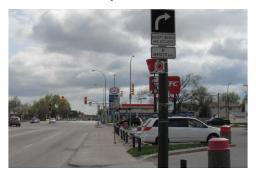
The mandatory turn for the right lane on McPhillips SB at Inkster is heavily enforced by police. This location only gives 25 m of advance warning for the upcoming lane drop which is just over 1 second for traffic traveling at the speed limit.
