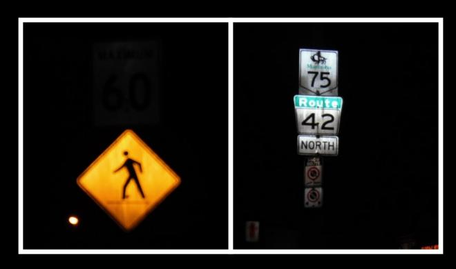
Speed limit signs should be as equally important as other signs. On many roads, every other sign is reflective except the speed limit sign. This includes route markers which serve very little safety purpose.
